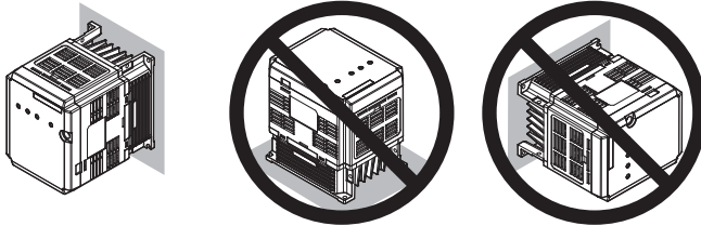
Figure 7 Correct Installation Orientation (Braking Unit)
